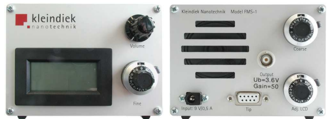
Front and rear panels of the FMS-LS controller provide visual and audio feedback and an analogue output
